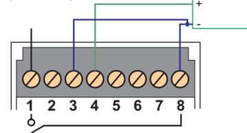
Thermocouple sensor, direct
