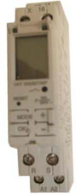
This timer has 14 programmable functions: 5 simple timer functions, controlled by the supply voltage and 7 functions controlled by separate control input. The timer is programmed directly on the front, and the LCD display will indicate the function and time during programming and operation.
