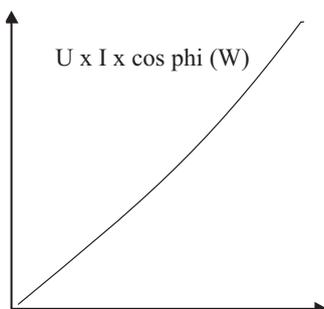
With power monitoring you can monitor all variables (supply voltage, current and phase angle), ensuring a very high sensitivity to even very small load changes, making this principle preferable for both over- and underload monitoring.
