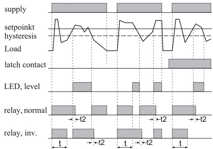
t = selected start-up delay, t2 = reaction delay
