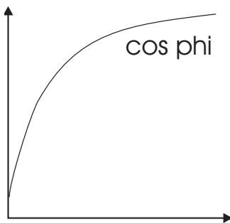
The phase angle between current and voltage ( $\cos \varphi$ ) is changing a lot between 0 and 60% load, therefore it is an advantage to monitor the phase angle if you want an alarm in connection with underload, f.inst. breakage of belts, pumps running dry, blocking of filters, etc.
